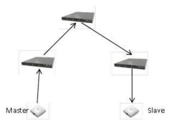
Note: In the lab, the IP base stations have successfully been synchronized with 5 enterprise LAN switches between master and slave.
